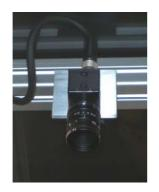
The camera detects the position and the orientation of the parts on the conveyor. The camera also distinguishes between LH and RH products (if applicable).
