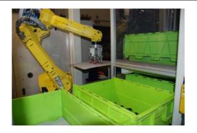
The machine allows to have a stack of intermediate sheets. Each time a layer has been completely finished, the robot will place one intermediate sheet.
