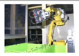
The robot places the products in a plastic case. If left hand (LH) and right hand (RH) products are moulded simultaneously, the robot distinguishes between LH & RH products: the robot takes one or several identical products (all LH or RH), and places them in the corresponding case (LH case, or RH case).
