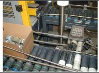
Once the case is filled, it is sent over the conveyor, through an inkjet printer (for marking the product ID) & case sealing unit.
