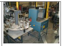
The robot presents the bundle to a cord strapping machine, and places the bundle in the corresponding case
