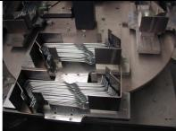
Unit that counts the wires & prepares bundles (one unit for each type of wire = for each standard production machine). The bundles are taken out by the handling robot.
