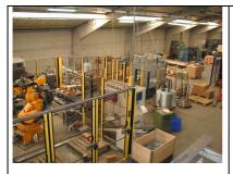
Case handling unit (consisting of a case erector, a case sealer, an inkjet printer and conveying equipment).
