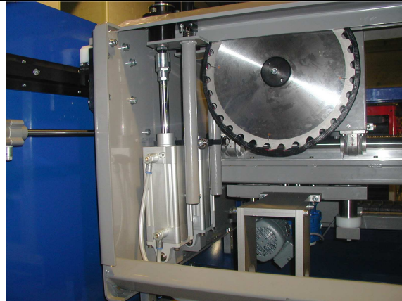
After each horizontal stroke, the circular saw moves up slightly (= vertical feeding stroke) until the full sheet thickness has been cut
