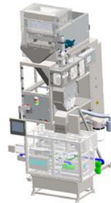
Can filling station (combined with a CTW250 weigher)
