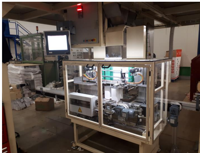
Can filling station (infeed conveyor to the left, outfeed conveyor to the right)
