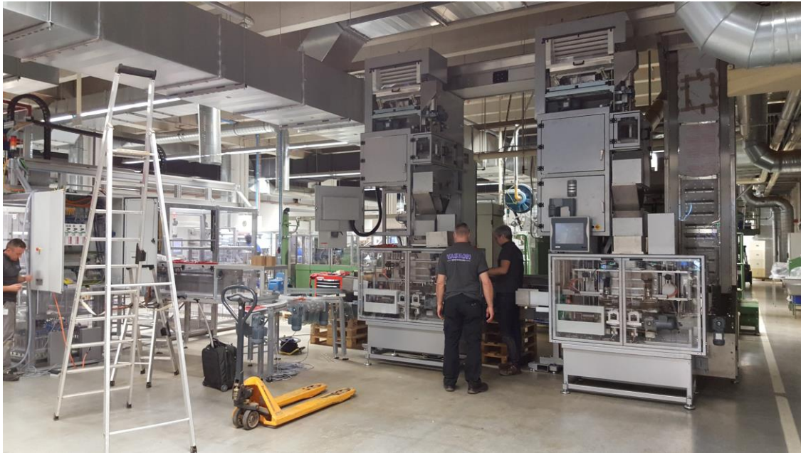
Combination of 2 tobacco weighers (CTW250), each having a can filling station. Empty cans are automatically destacked from pallet (option "destacker for empty cans").
