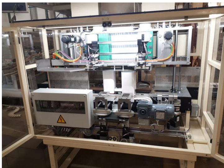
Can filling station (infeed conveyor to the left, outfeed conveyor to the right)
