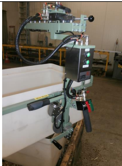
Operating unit allows to turn the box upside-down
