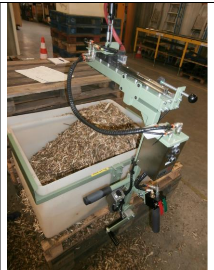
typically used to empty tobacco in a feeder (feeding a packaging line)
