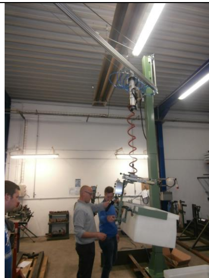
Ergonomic lifting of box (29kg)
