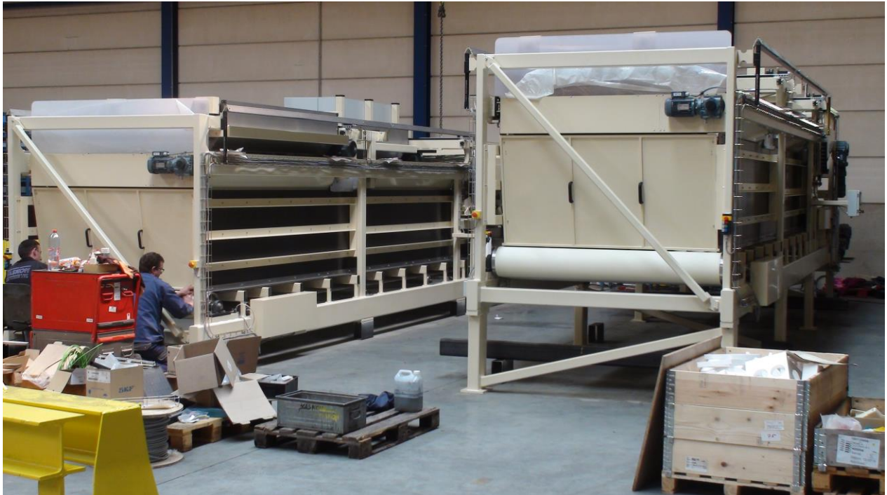
2 high capacity Straight layers (capacity of each machine : 2.500 kg of tobacco leaves/h)
