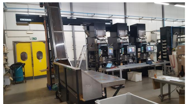
3 weighers combined in one line With option "control of feeder conveyor" With option "Central control System"
