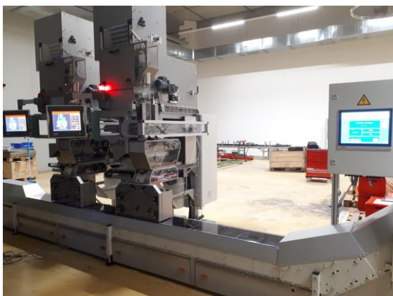
2 weighers combined in one line With option bucket chain conveyor / CCS
