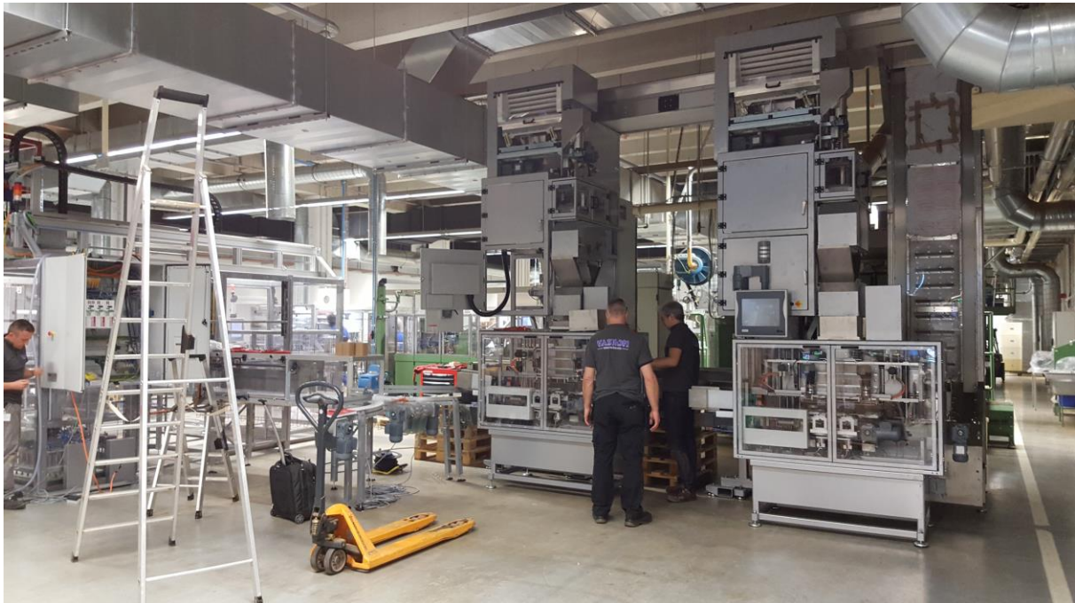
Weigher CTW250 (2x) for filling cans with tobacco In this particular layout, the weighers are combined with the optional can filling station (2x) + with the optional "destacker for empty buckets"
