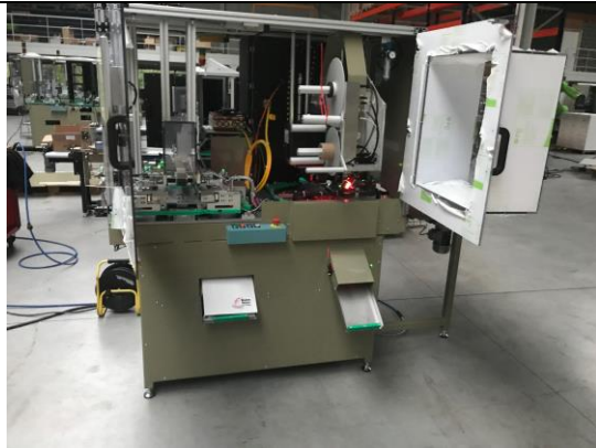
Track & trace : laser coding of individual pouches + coding of bundles
